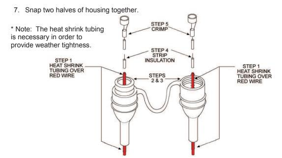
Figure 4: Fuse Holder Assembly
